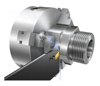
tougher insert grades without the risk that they might collapse from the combination of high temperature and high force on cutting edge and corner radii – so-called plastic deformation. This provides the basis for more predictable tool life and a more secure machining process.
