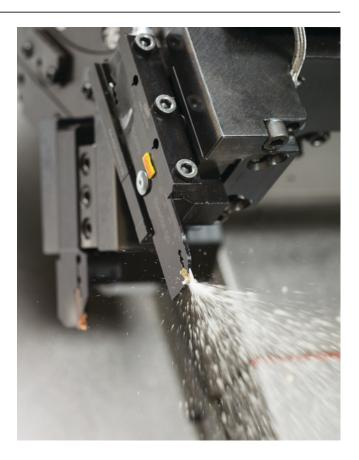
coolant delivered with precision that helps impact the exact cutting zone (the point of contact between insert and workpiece), penetrating into spaces and grooves where it can make a real difference to machining.
