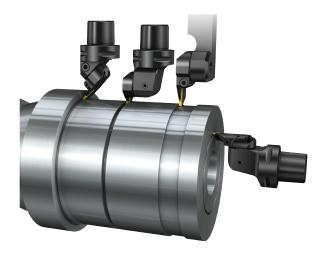
reduces temperature in the cutting zone and improves chip evacuation. When external coolant is applied conventionally in parting and grooving, the amount of coolant that actually gets into the groove is very small, and the effect is minimal, especially when machining deep grooves. However, with qualified, high precision, high pressure coolant application, accurately directed jets properly access the cutting edge, even in deep grooves.
