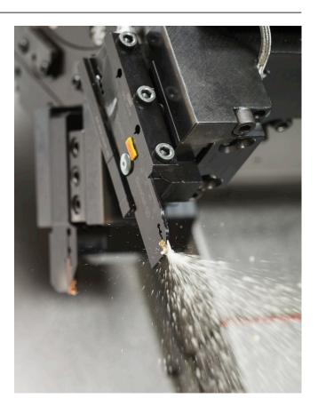
coolant delivered with such precision that it impacts the exact cutting zone (the point of contact between insert and workpiece), penetrating into spaces and grooves where it can make a real difference to machining.
